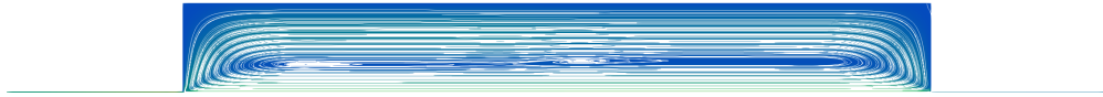
Figure 5.48: Slice of the velocity field with streamtraces for y = 0.005 m for the sliding hydrostatic bearing.
