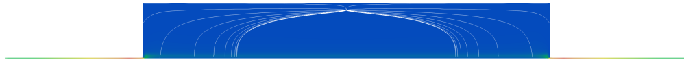
Figure 5.35: Slice of the velocity field with streamtraces for y = 0.011 m for the hydrostatic bearing without motion.
