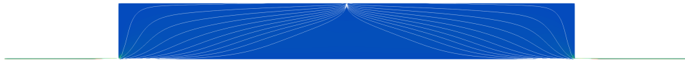
Figure 5.34: Slice of the velocity field with streamtraces for the y = 0.009 m for the hydrostatic bearing without motion
