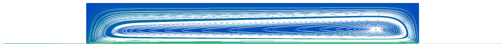
Figure 5.50: Slice of the velocity field with streamtraces for y = 0.009 m for the sliding hydrostatic bearing.
